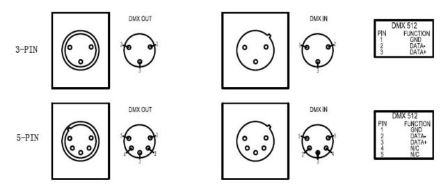
Connection between the controller and a projector and between one projector and another must be made with a 2 core-screened cable, with each core having at least a 0.5mm diameter. Connection to and from the projector is via cannon 3 pin (which are included with the projector) XLR plugs and sockets. The XLR's are connected as shown in the figure above.
